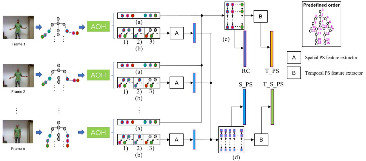
Figure 2: The illustration of PS features extraction (T\_PS, S\_PS and T\_S\_PS). (a) and (b) are single joints and joint pairs selected following AOH. (c) and (d) are the temporal paths of single joint and each dimension of S\_PS. Note that TTM (proposed in Section 4.2 and illustrated in Fig. 4) should be implemented between AOH and PS extractors, but we omit it here for clarity.
