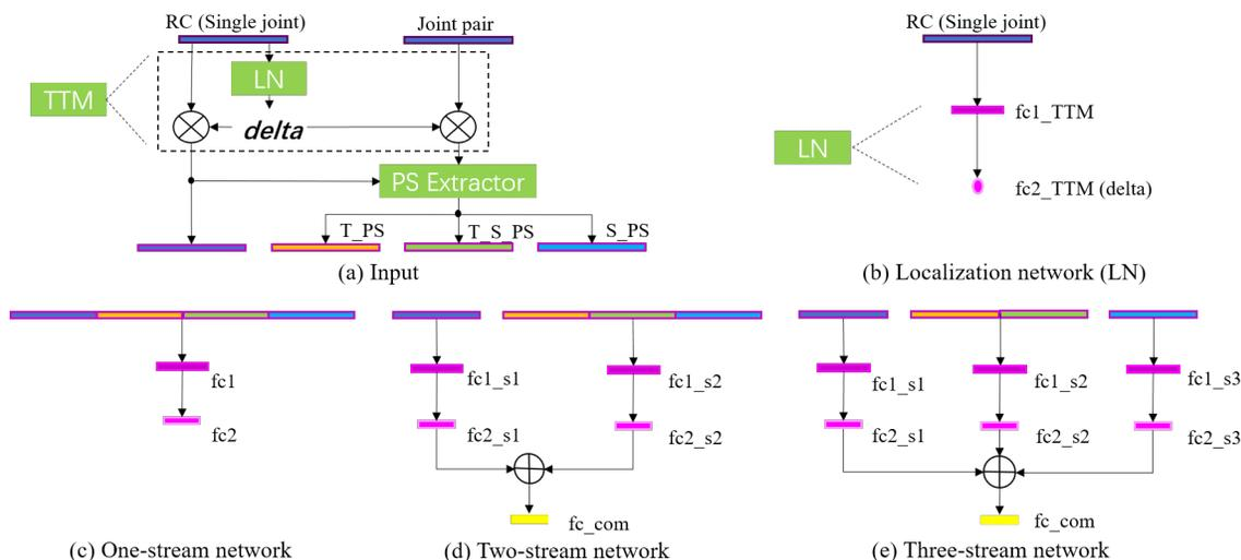
Figure 4: Three different types of network architectures: one-stream network (1s\_net), two-stream network (2s\_net) and three-stream network (3s\_net). TTM is the temporal transformer module. LN is the localization network that generates the transformation parameters  $\Delta$ .  $\otimes$  and  $\oplus$  denote temporal shift and weighted sum. The fc2 in each stream denotes a FC layer with a softmax activation function.
