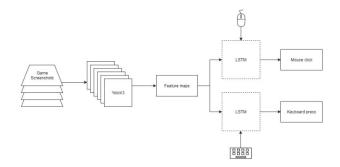
Figure 2: LSTM Architecture
