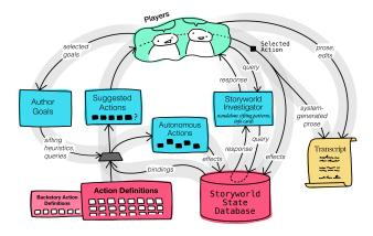
Figure 2: An overall system diagram of *WAWLT*, showing the important modules and data flows. Pink subsystems (action definitions and the storyworld state database) consist of inert data; blue subsystems (author goals, suggested actions, autonomous actions, and the storyworld investigator) act on this data; and the transcript emerges from player actions over the course of play.
