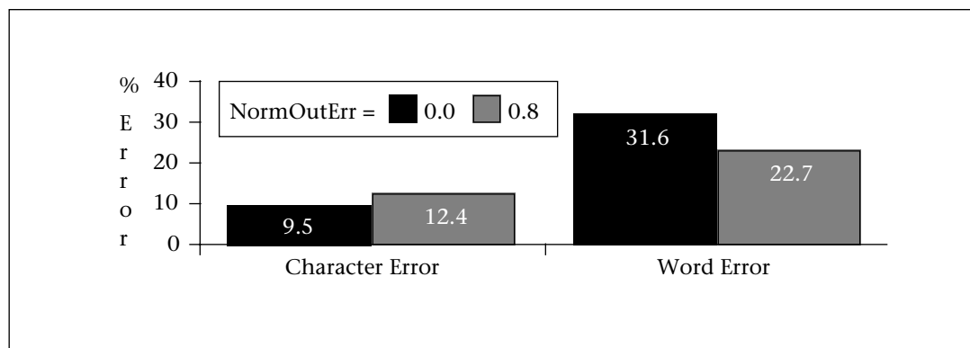
Figure 5. Character and Word Error Rates for Two Different Values of NormOutErr (d).
