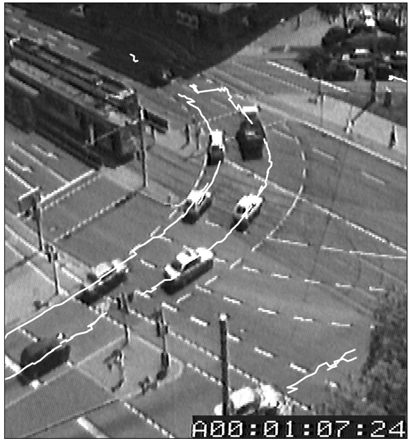
Figure 5. Vehicle Trajectories Obtained by Tracking Clusters of Feature-Based Optical Flow Estimates. (From Otto [1990]).
