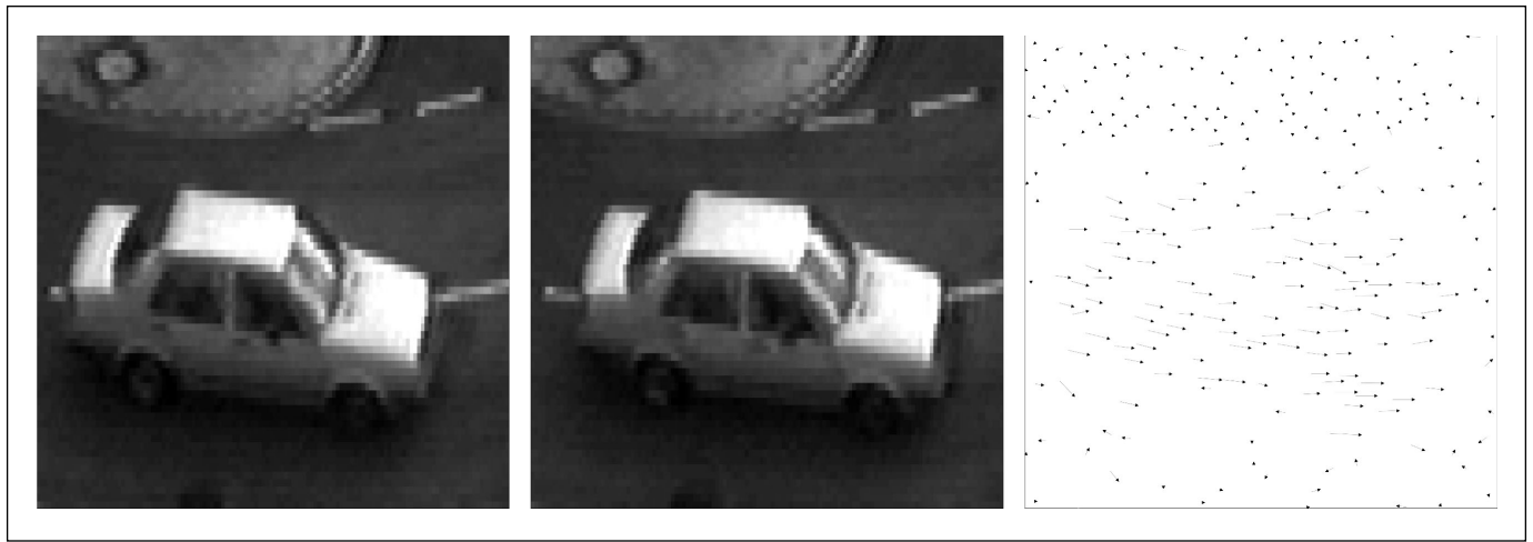
Figure 3. Feature-Based Optical Flow Results (Right Panel) Estimated from Image Regions (Left and Center Panels) That Have Been Cropped from Two Frames of a Sequence.
