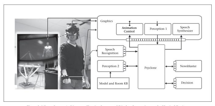
Figure 2. Mirage System Architecture, Showing Sensor and Display Connections to the Physical Devices. Arrows to and from Psyclone indicate message and control flow. Small striped rectangles on the edges of modules signify Psyclone adapters.
