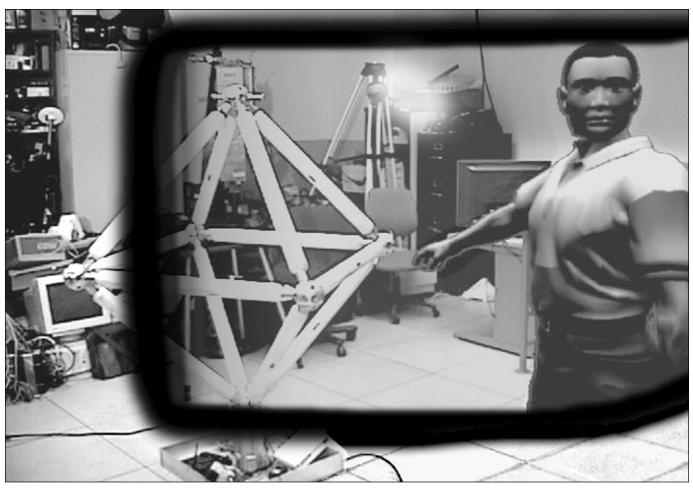
Figure 1. Our Embodied Agent Mirage Is Situated in the Laboratory. Here we see how Mirage appears to the user through the head-mounted glasses. (The image has been enhanced for clarity.)
