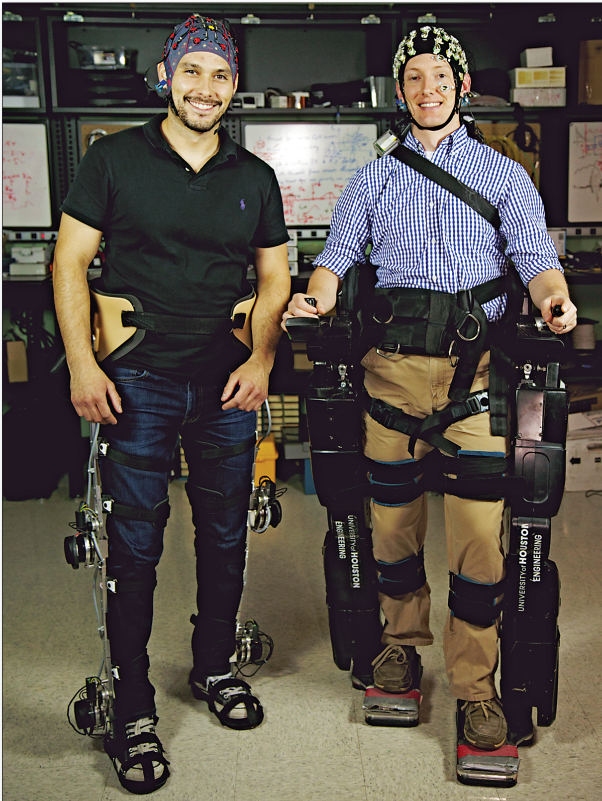
Figure 1. Two Examples of Exoskeletons with Bilateral Powered Ankle, Knee, and Hip Joints.
