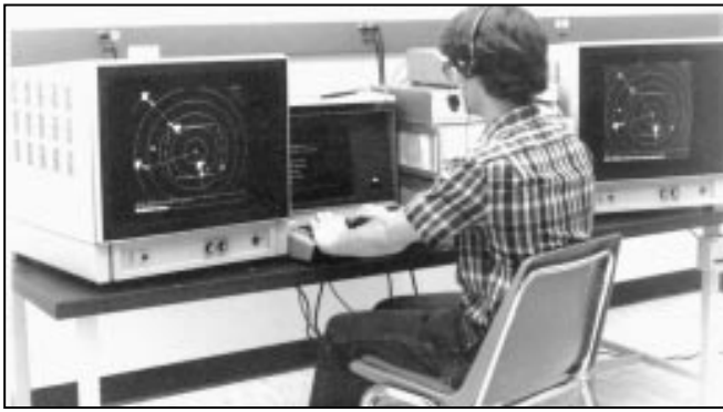
Figure 5. The Two Displays of the Predictive Man-Machine Environment System Showing Simulated Radar Scopes.
