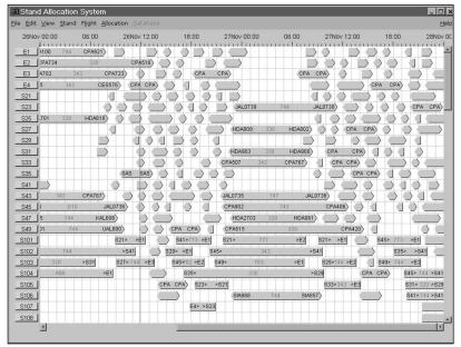
Figure 1. sas Gantt Chart with Two Days of Assignments.
