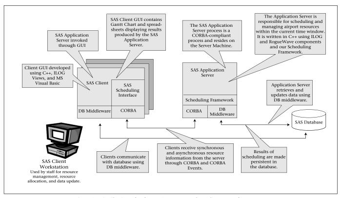
Figure 8. Distribution of Software Components through CORBA Infrastructure.
