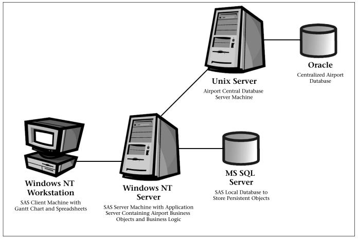
Figure 3. The sas Hardware Architecture.
