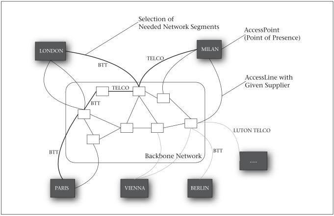
Figure 1. Reseller's View on IP-VPN Network.
