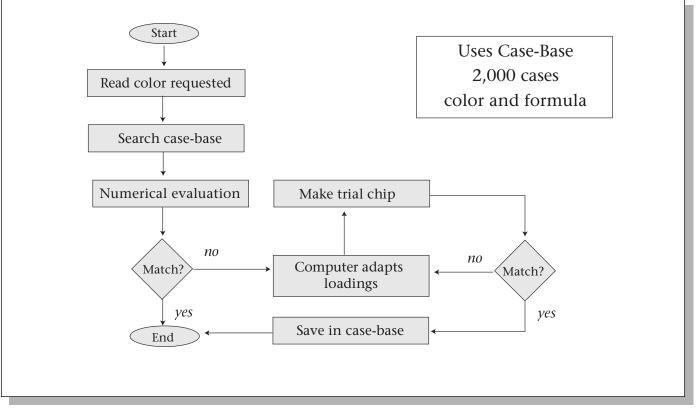
Figure 3. The Automated Color-Matching Process.
