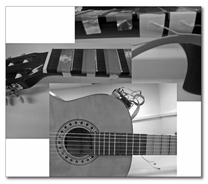
Figure 4. Nonintrusive Capacitive Sensors Mounted on the First 10 Frets of a Nylon Strings Guitar.
