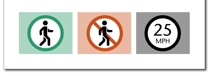
Figure 2. Proposed Displays to Aid Pedestrians in Making Road Crossing Decisions in the Presence of Self-Driving Cars.
