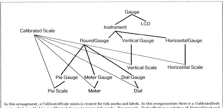
In this arrangement, a CalibratedScale mixin is created for tick marks and labels. In this reorganization there is a *CalibratedScale* mixin which is added to uncalibrated classes to create tick marks. For example, *VerticalScale* is a subclass of *VerticalGraph* and uses the *CalibratedScale* mixin.
