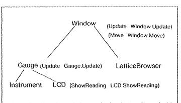
In hierarchical inheritance in Loops, the description of a method is inherited by every subclass, unless it is overridden in the subclass. This inheritance can be characterized as a *first-found* search through superclasses. In this figure, the Move method for the class *LCD* is inherited from *Window*.
