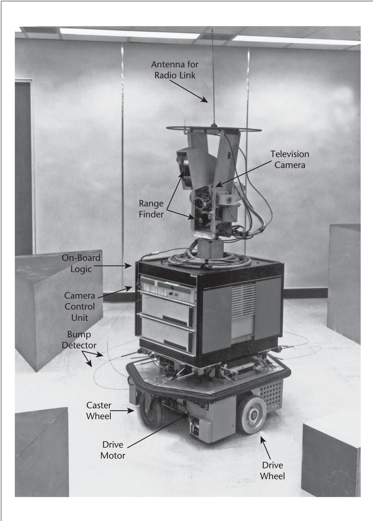
Figure 3. Shakey the Robot.
